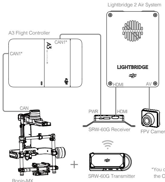
\*You can connect the CAN cable to the CAN Hub on the GPS cable.
