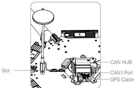
⚠ • Ensure that the GPS module is securely mounted and the arrow is pointing towards the nose of the aircraft.
