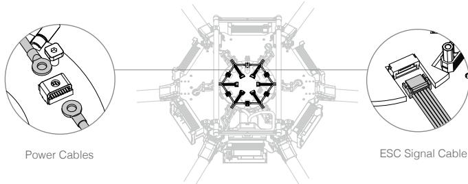
9. Ensure that all ESC cables and power cables are correctly installed on the center frame.
