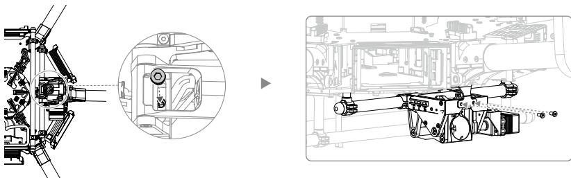
5. Insert and tighten the four M3×6.5 screws to secure the retractable module on the mounting rod.
