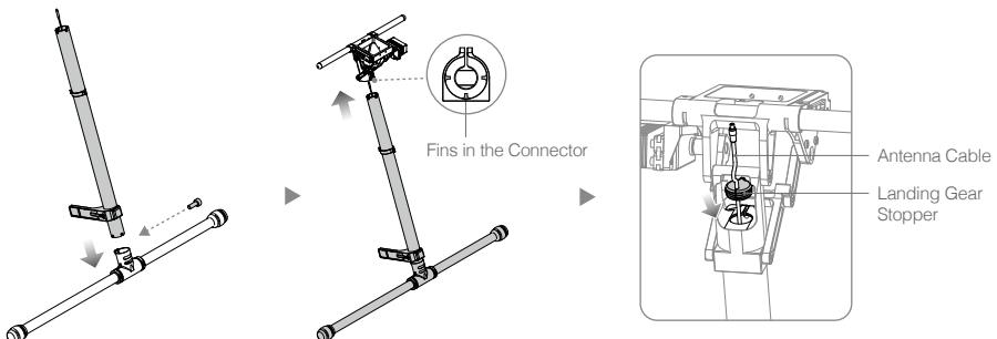
4. Insert two M3x8 (cylinder) screws into the screw holes on the connector and tighten. Be sure to insert the screws from left to right as shown below to avoid damaging the screw holes.
