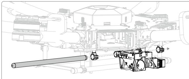
3. Align the cable fixing ring and the screw hole on the bottom of the retractable module. Insert and tighten the M3×5.5 screw.
