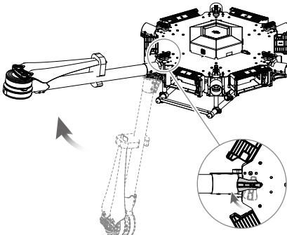
7. Connect the power cables to the center frame. Each cable must be screwed into a positive (+) or negative (-) gold bracket. Red cables are positive and black cables are negative. Each bracket will have two cables of the same color screwed into it. Then tighten each M3×5.5 screw (square head) using the square socket wrench.
