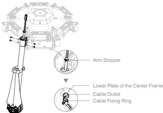
6. Gently lift the frame arm. Twist the red knob to lock each arm in place. Be sure you hear an audible click, which indicates a proper lock. Check the arm for movement. To store, untwist the knob and lower the frame arm.
