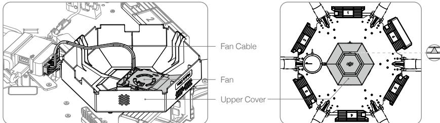
⚠ DO NOT damage the fan cable when removing the upper cover of the center frame.
