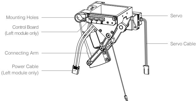
1. Mount the retractable module bracket to the mounting position on the lower plate of the center frame as shown below. Apply medium strength threadlocker to two M3x8.5 screws. Insert and tighten the screws.
