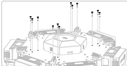
2. Mount the four brackets of the expansion bay to the upper plate of the center frame by inserting and tightening twelve M3x8 screws.
