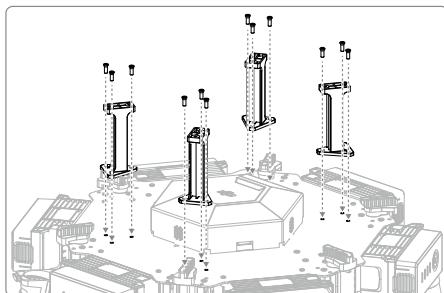
3. Mount the base plate of the expansion bay to the brackets by inserting and tightening eight M3x5.5 screw.
