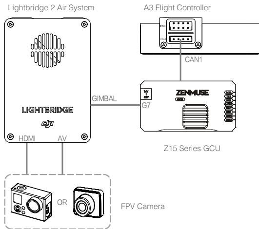
When using the Zenmuse X3, X5 Series, XT or Z15 series HD gimbal, set the App Output Mode in the DJI GO app to display the image on your mobile device from the camera used with your gimbal. Launch the DJI GO app > Camera View > **HD** > Enable EXT Port, adjust the Bandwidth Allocation to ensure that the "EXT" percentage is more than 0%, and then set the App Output Mode to EXT.
