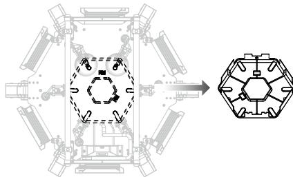
3. Insert the frame arm into the arm connector on the center frame with the propeller away from the center frame. Rotate the frame arm to align the screw holes on the frame arm and connector. Then insert and tighten four M3×6.5 screws.
