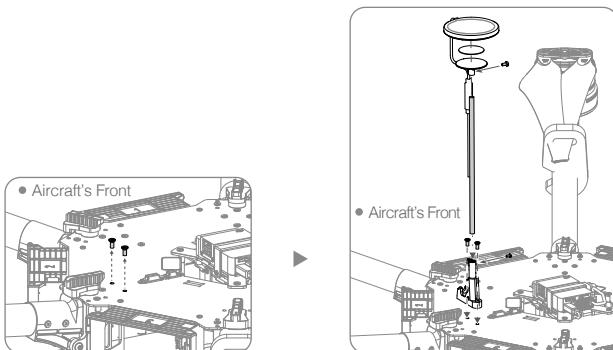
4. Plug the GPS cable into the CAN1 port on the flight controller.
