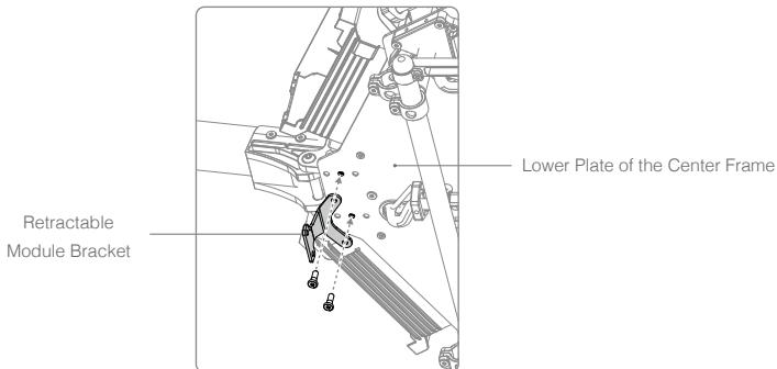
2. With the servo of the retractable module at the rear of the aircraft, insert the retractable module mounting rod into one mounting hole on the center frame, mounting holes on the retractable module and the other mounting hole on the center frame respectively. Ensure that the left retractable module is mounted on the left side of the aircraft (when viewed from the rear).
